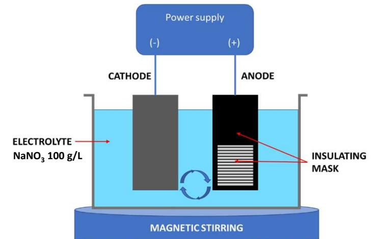
→ 180 s galvanostatic polarization set at  $2 \text{ A}/\text{cm}^2$
