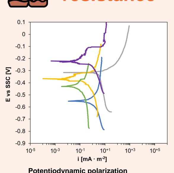
**Potentiodynamic polarization** 20 ppm Cl<sup>-</sup>, 1 h immersion
