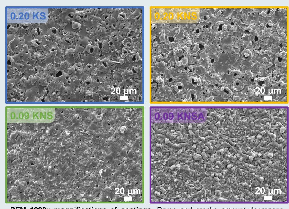
SEM 1000x magnifications of coatings. Pores and cracks amount decreases with spark intensity.
